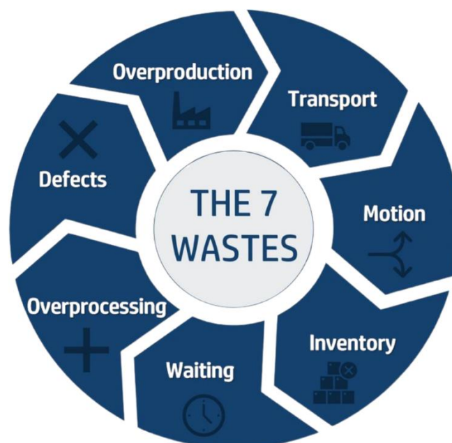
Fig. 1. The seven types of waste within Lean manufacturing Source: "7 Types of Waste in Lean Manufacturing", 2021
